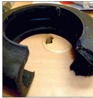
Horizontal coupling used vertically Over Loading/Loose Clamping
