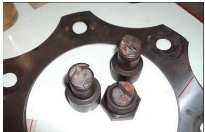
Incorrect Selection / Incorrect Installation
