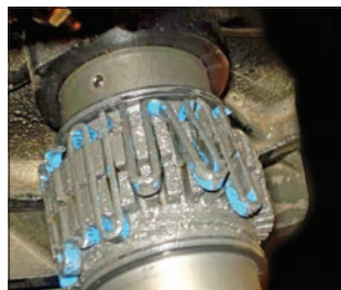
Undersize Coupling for Application
