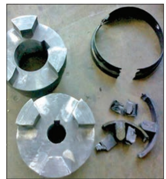
Mis-aligned coupling - Vibration beyond limits
