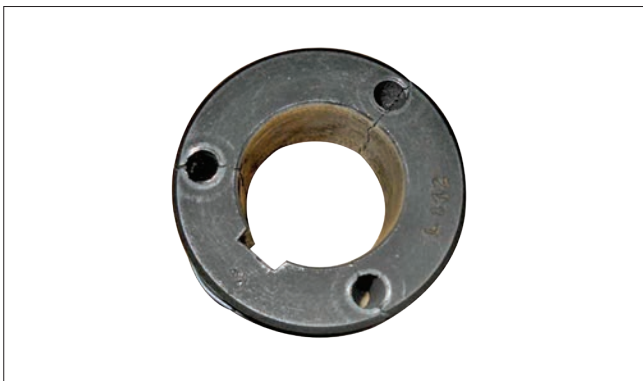
- Excessive Interference Fit: Hub Cracked at 3 Holes
