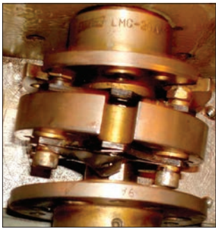
Horizontal coupling used vertically Over Loading/Loose Clamping
